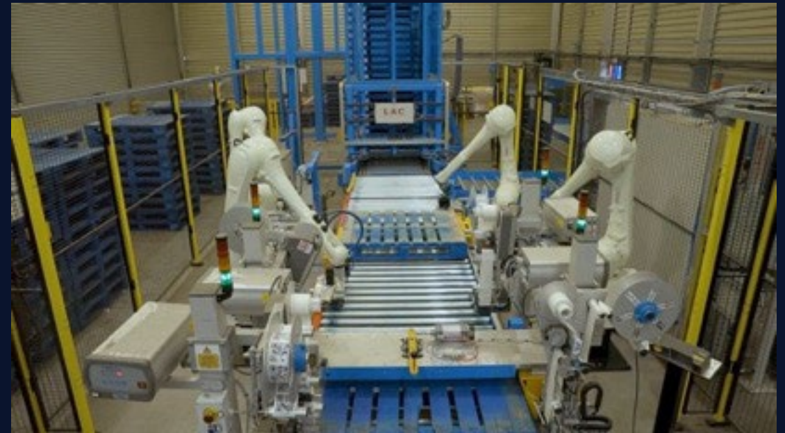
Automatic tagging robot attaching QR Codes in Birmingham UK, validating operational feasibility proven in Chile
