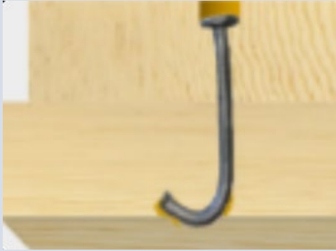
Clinch nails in repair
